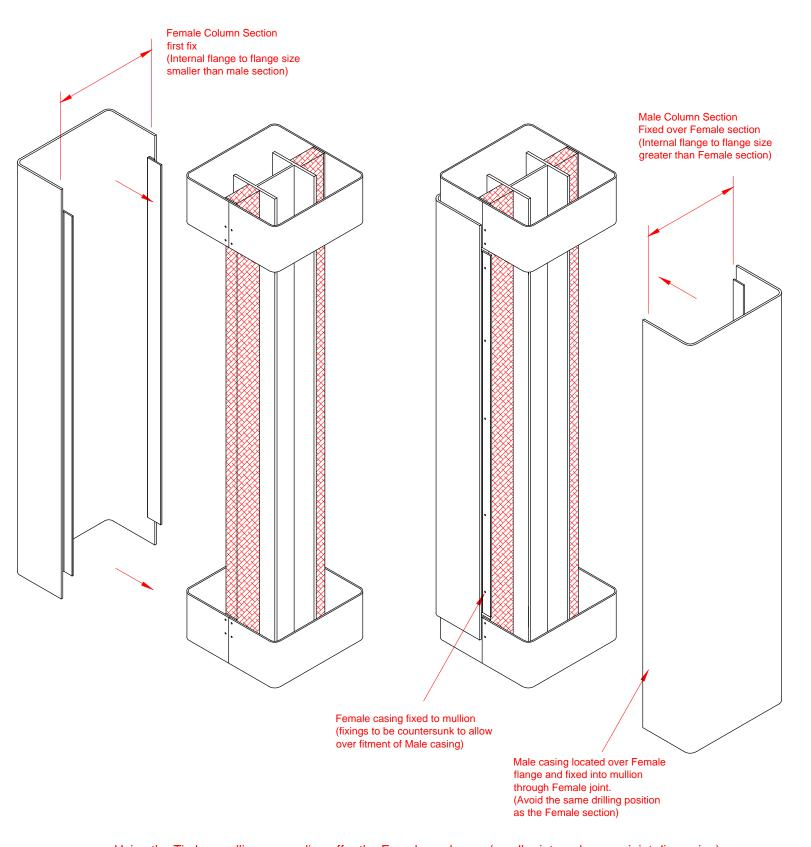
Using the Timber mullion as a spline offer the Female enclosure (smaller internal across joint dimension) so that the required amount of inner collar is revealed. Screw through the joint and into the mullion. Countersunk screws are required for this first section as the second section locates on top of the flange.
