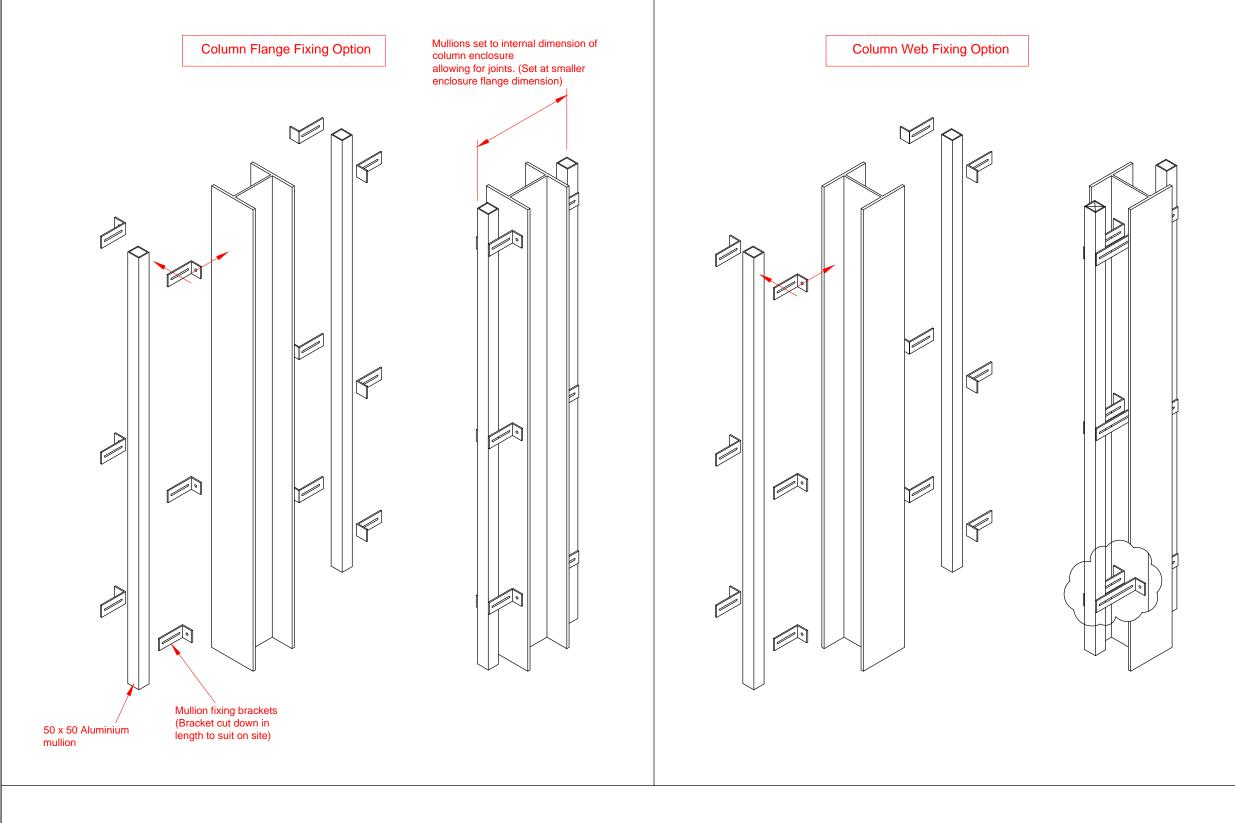
Fix the 50 x 50 aluminium mullion to existing column to suit internal dimensions of column enclosure
